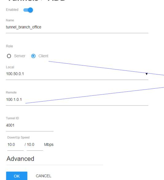
It is required to type in the remote IP when the tunnel is in client role.
